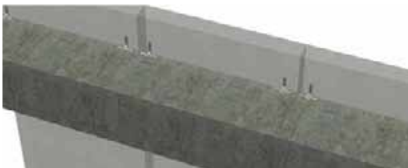
Example of anchoring between the vertical panels and flat roof beam.
