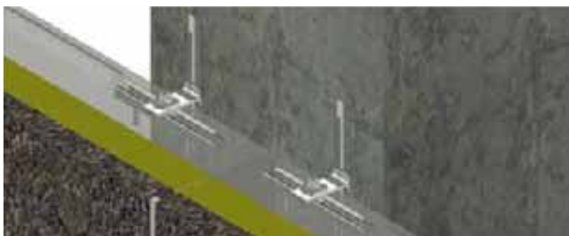
Example of anchoring between the horizontal panels and pillar.
